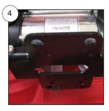
Attach metal base plate to side of pump. This will be to secure nozzle holster
